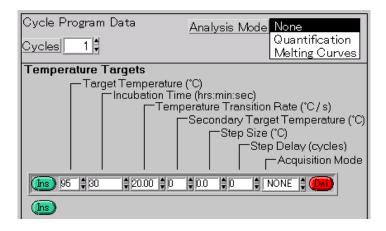
(2) The cycling parameters should be set according to the following window. Analysis mode of the PCR step must be set at "Quantification". Acquisition modes of 95°C and 60°C must be set at "None" and "Single", respectively.
